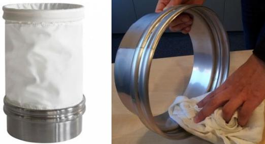
Avoid using sharp objects to remove the BFM® connector from the spigot as these may damage the connector material. Regularly check and clean the inside of the ring profile of the BFM® spigot to remove e.g. product residue.
